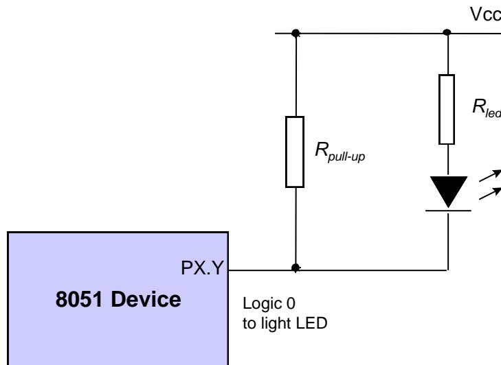
The value of the pull-up resistor should be between 1K and 10K. This requirement applies to all of the examples on this course.
