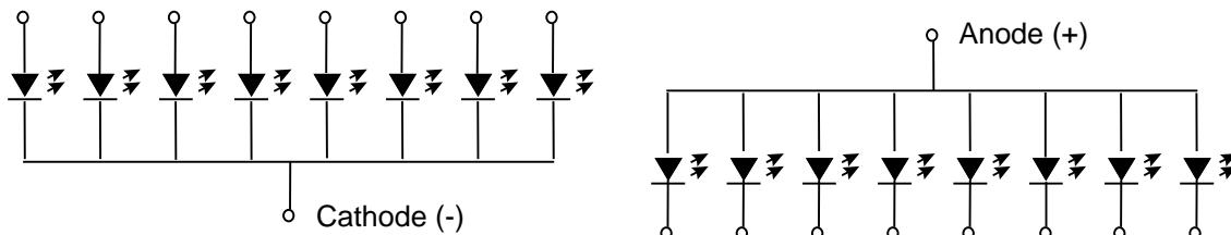
The required current per segment varies from about 2 mA (very small displays) to about 60 mA (very large displays, 100mm or more).
