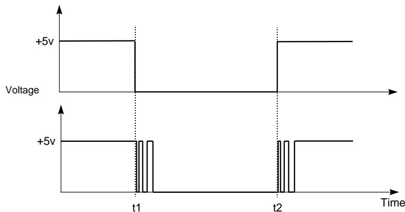
As far as the microcontroller is concerned, each ‘bounce’ is equivalent to one press and release of an ‘ideal’ switch. Without appropriate software design, this can give rise to a number of problems, not least:
