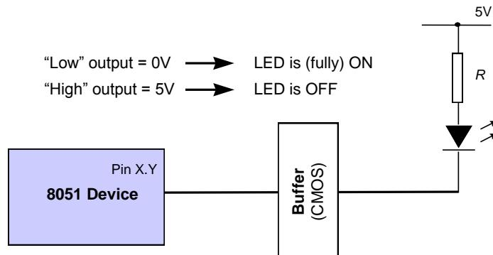
*Using a CMOS buffer.*
