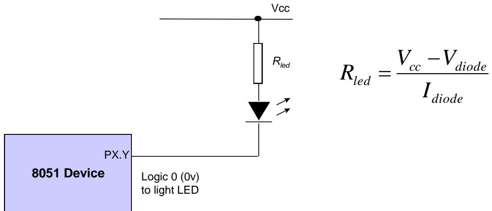
Connecting a single LED directly to a microcomputer port is usually possible.
