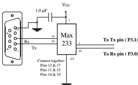
*Using a Max 233 as an RS-232 transceiver.*
