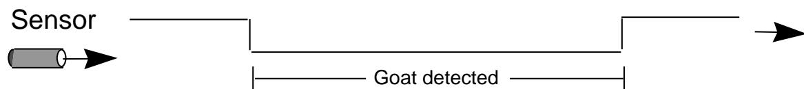
If we try to use the code in the previous example, **the goat sensor will not allow us to count the number of goats but will instead provide an indication of the time taken for the goats to pass the sensor.**
